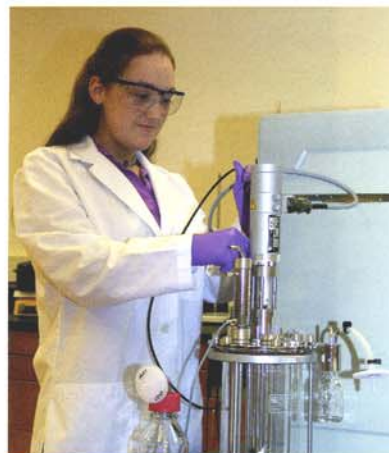
NHCTC student assembling a bioreactor for CHO cell culture that will produce the clot-buster, tPA
